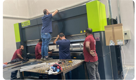
CNC press brake commissioning
